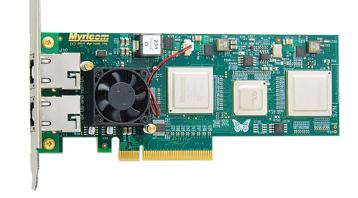
**C-Class** – This is our cost-optimized series. It is 10 Gbit only and comes in one or two port versions. There are several form factors including: PCle low profile, IBM BladeCenter, and an industrial/defense optimized PC/104. The C-series supports both Windows and Linux.
