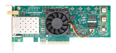
E-Class – This is our feature-oriented series, while still cost optimized. It supports both 1 Gbit and 10 Gbit, 2-port and 4-port. It is PCIe low profile only. There are hardware assists for both merging and RSS to reduce CPU overhead below even the C-Series benchmark. The accuracy of the E-Series timestamps equals that found on much more expensive boards. E-Series is currently Linux only.
