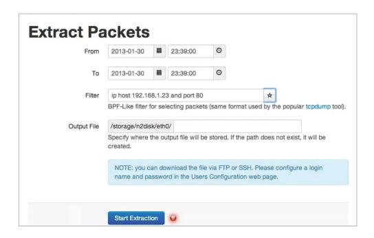
The user interface simple and powerful specification of packets to be extracted based on capture time and or BPF-like filtering.
