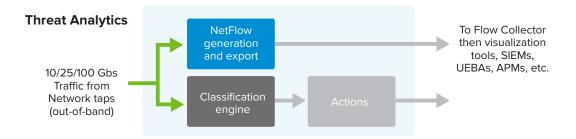
ARIA NSS can also shunt certain flows, such as streaming video and audio-only, sending a specified number of bytes for inspection. Such adaptive filtering allows detection tools to operate more effectively by only analyzing the most relevant traffic. For SIEMs like Splunk and QRadar that charge by ingested bit, this translates into dramatic cost savings.
